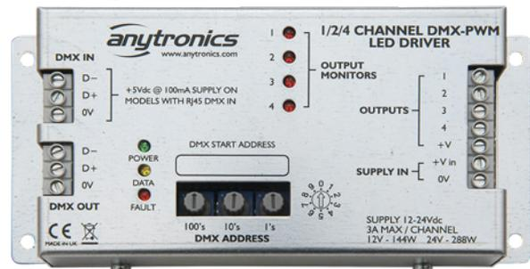
The Anytronics DMX to PWM LED driver provides four controllable PWM outputs for controlling LED loads connected with common anodes to a single supply in the range 12-24V DC. Where necessary, multiple supply configurations are also possible provided that the unit is also powered from the highest supply voltage in the range 12-24V. (See overleaf).
