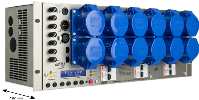
Series 194 D612 - 6 x 12A Dimming / Switching with On Board Level Controls (OBLC) 12 x 16A CEE17 sockets and 2 DMX inputs
